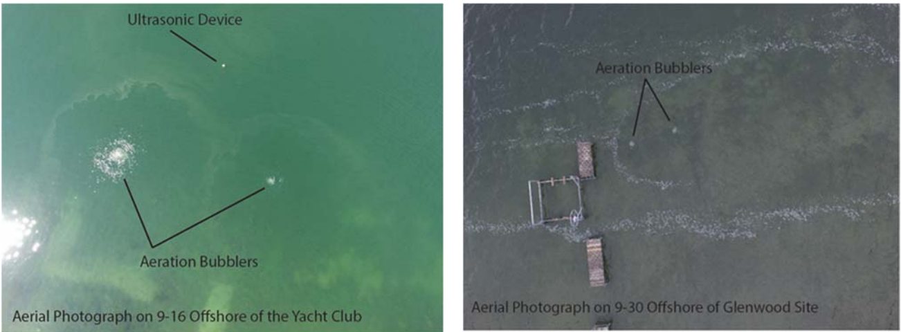
Fig. 11. Drone images revealing circular BGA rings at the Yacht Club and Glenwood Rd. BGA mitigation sites.
